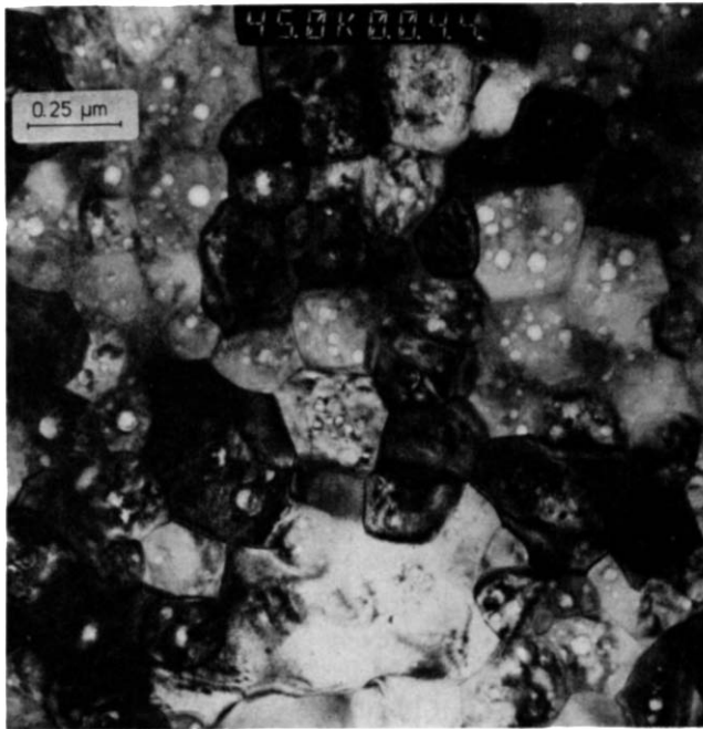
Fig. 9. TEM micrograph of sintered (1260°C in air) hydrothermal BaTiO 3 showing intragranular porosity.
